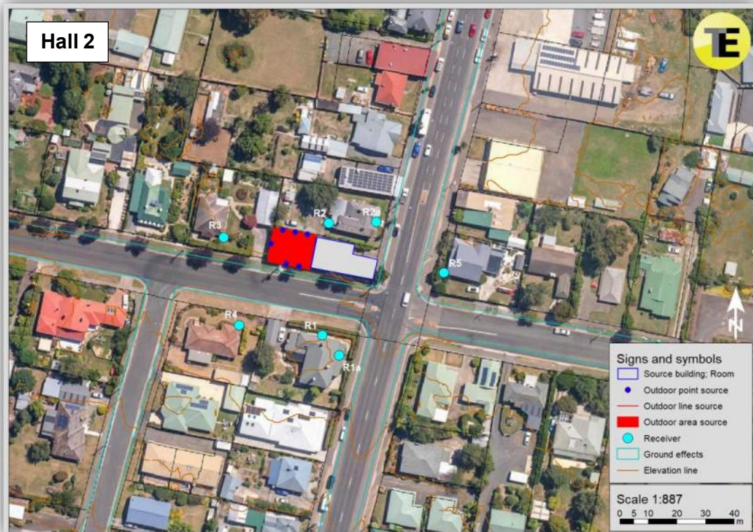
Figure 5-1: Environmental noise model plan view, amplification noise .
