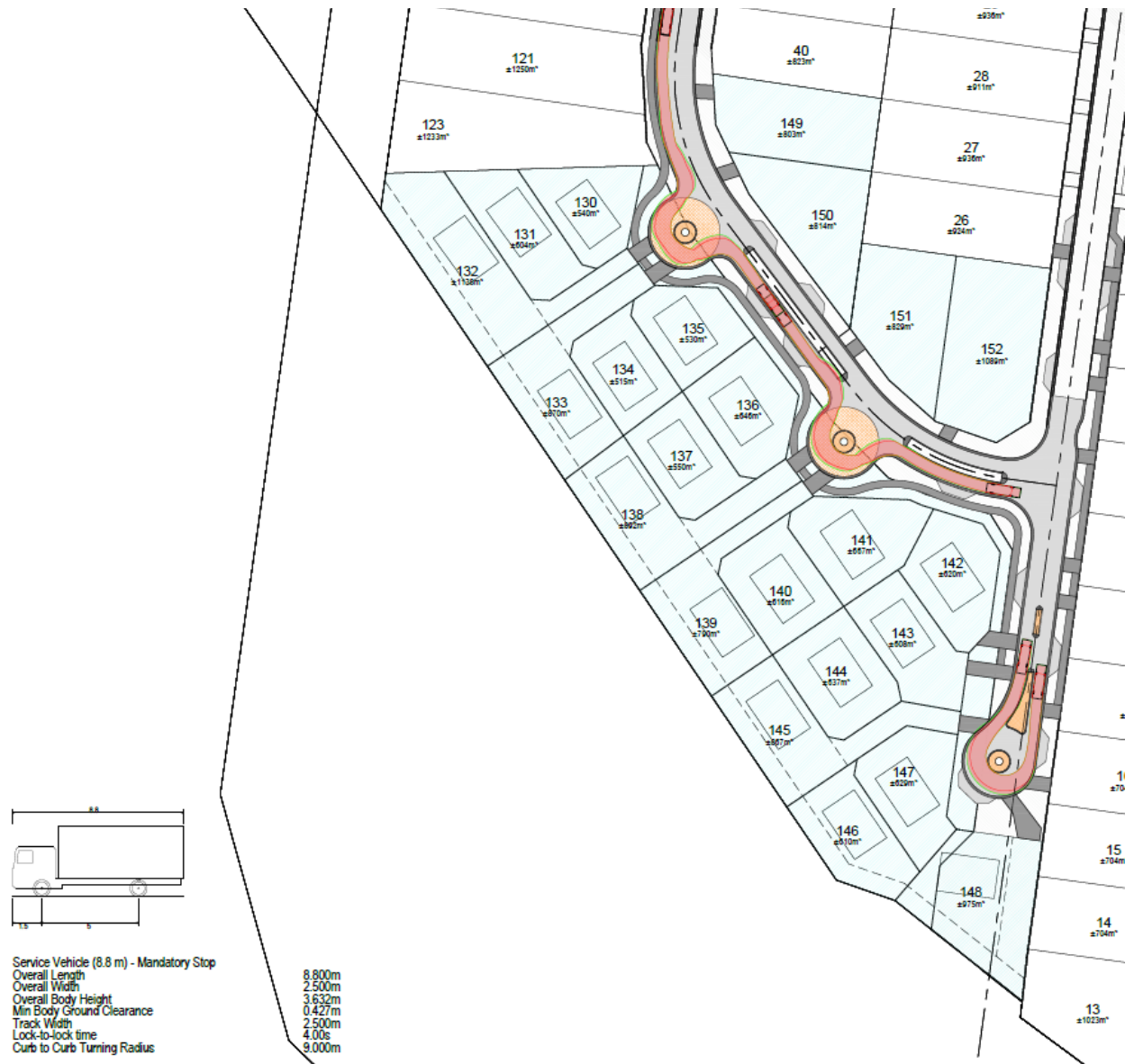
Figure 3c – 8.8m Medium Rigid Vehicle turn path checks
