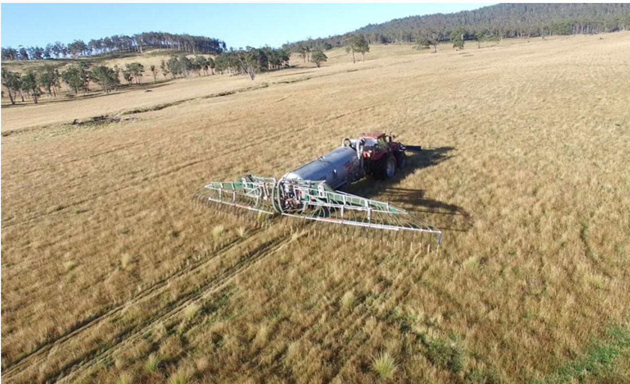
Figure 4: Typical spreader arrangement. Photo shows a Pichon 20700 litre vacuum spreader and 335hp 4WD tractor, taken at St Peters Pass Oatlands 2021
