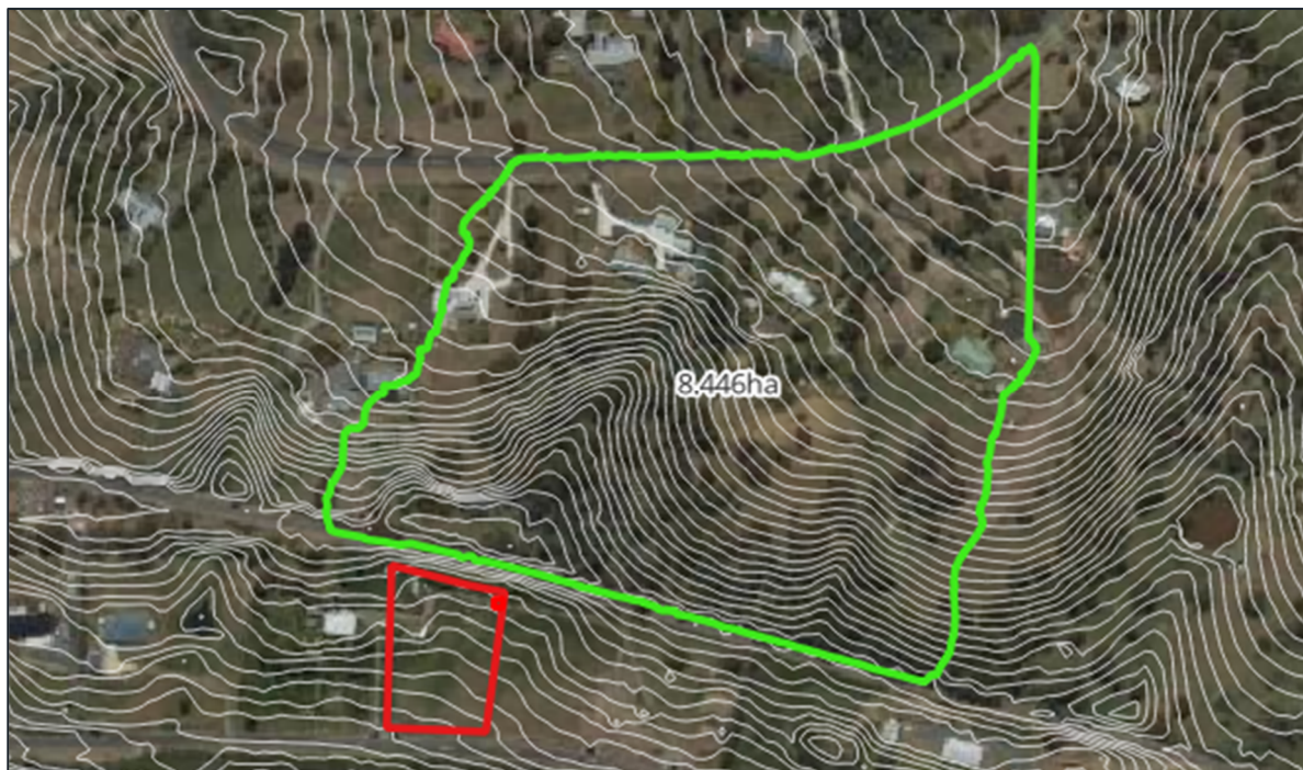
Figure 3. TasRail Culvert (KPW 021.777) Catchment Area
