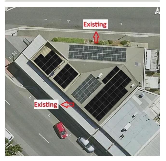
**Existing Solar System** - Site has an existing solar system of 13.2Kw capacity. Existing system associated with the lighter ( Grey ) colour as mentioned above in the site plan.
