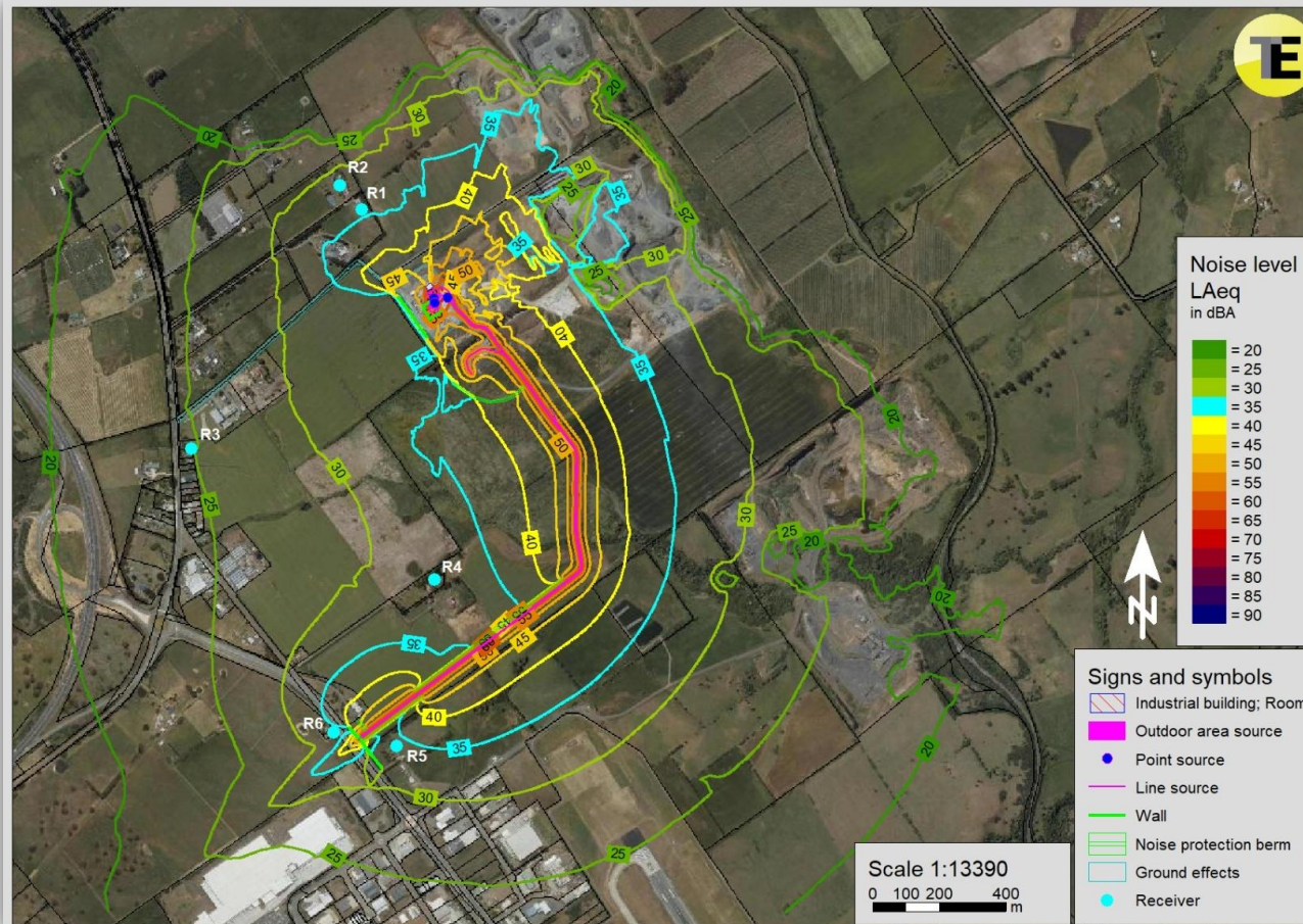
Figure A-6: Predicted L_{Aeq} contours under CONCAWE worst-case weather, Combined operations
