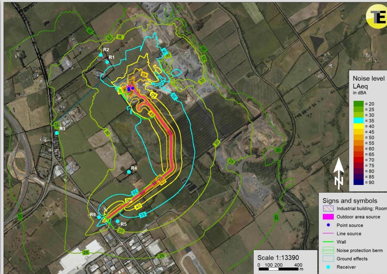
Figure A-5: Predicted L_{Aeq} contours under ISO, Combined operations .
