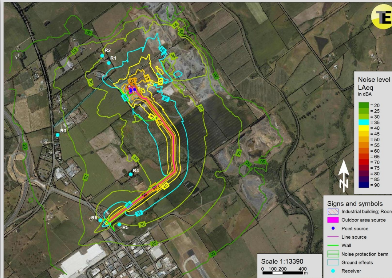
Figure A-1: Predicted L_{Aeq} contours under ISO, Batch Plant operations .
