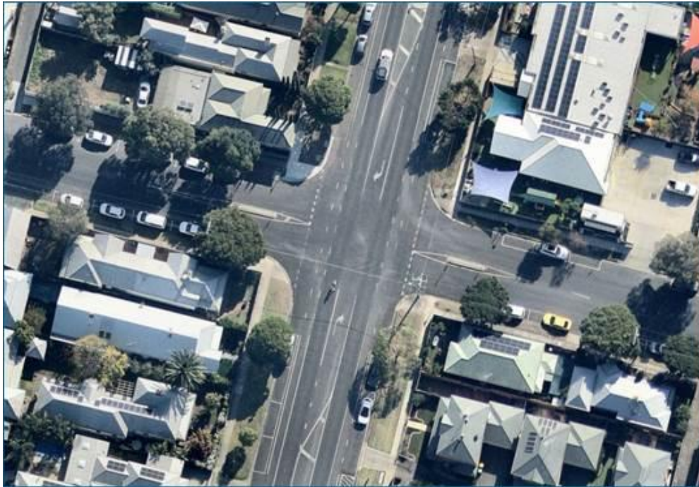
Figure 7.14: Basic right-turn treatment (BAR) for a two-lane urban road
