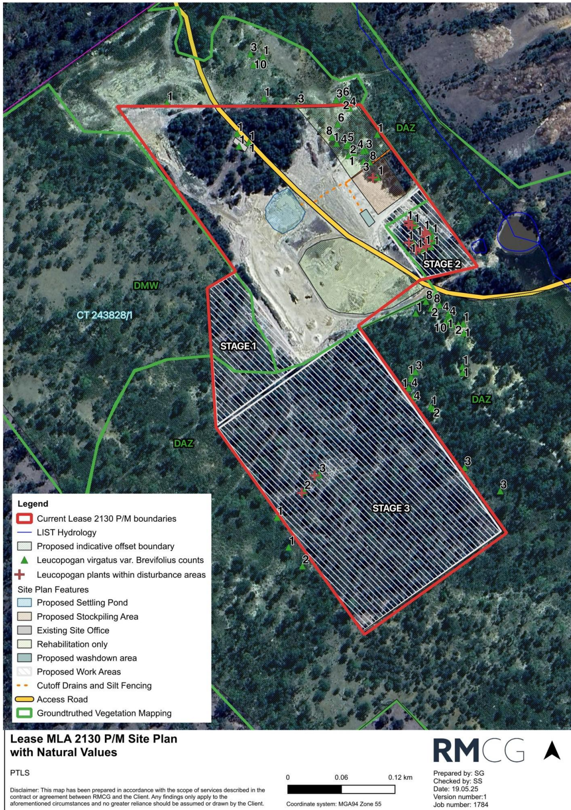
Figure 4. Site Plan with Natural Values (Appendix A, Figure A2-4). Note records of Leucopogan virgatus var. brevifolius to be marked on site and avoided.
