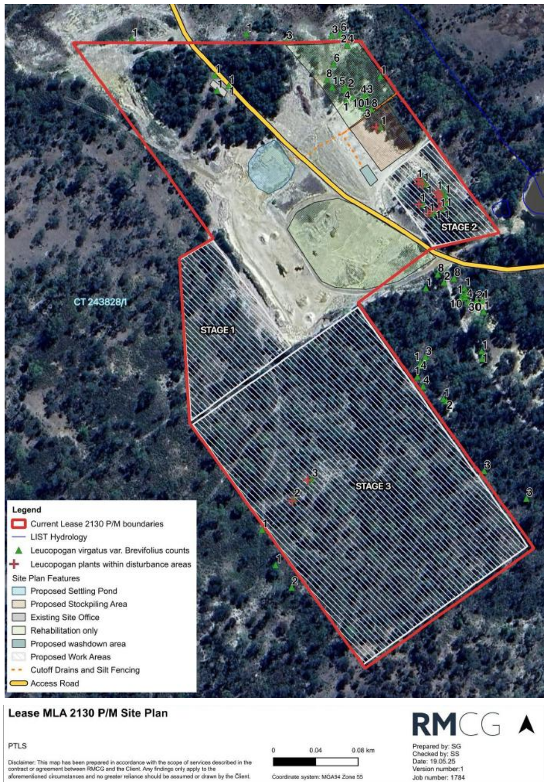
Figure 3: Site plan showing the locations of Stage 1, Stage 2 and Stage 3 extractive areas and site infrastructure. Activity Area and mining lease 2130P/M boundaries are shown in red and are inclusive of the proposed extractive pit expansion area (Figure 3 of the EER).
