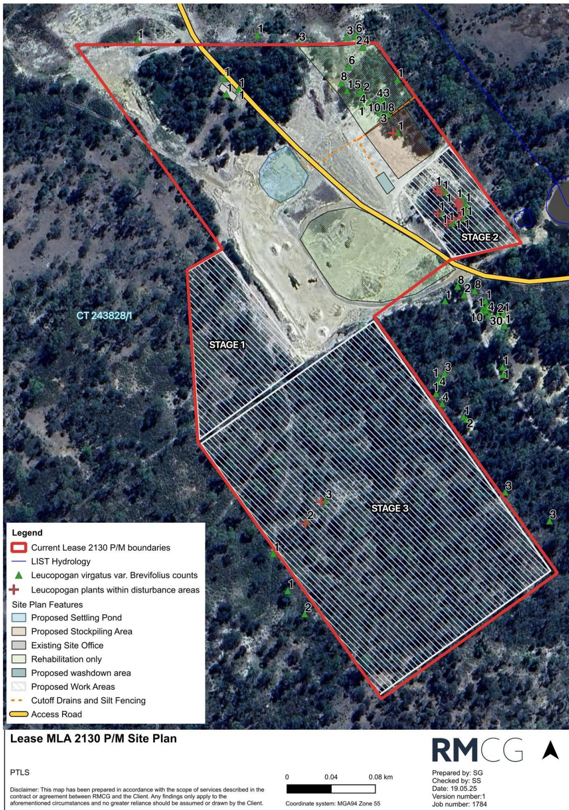
Figure 3. Lease 2130P/M Site Plan defines the area on which the activity will take place. It also shows the location of existing workings, proposed working areas, existing roads, areas currently under re-habilitation, locations of threatened species, water management (including settling pond) and watercourse.
