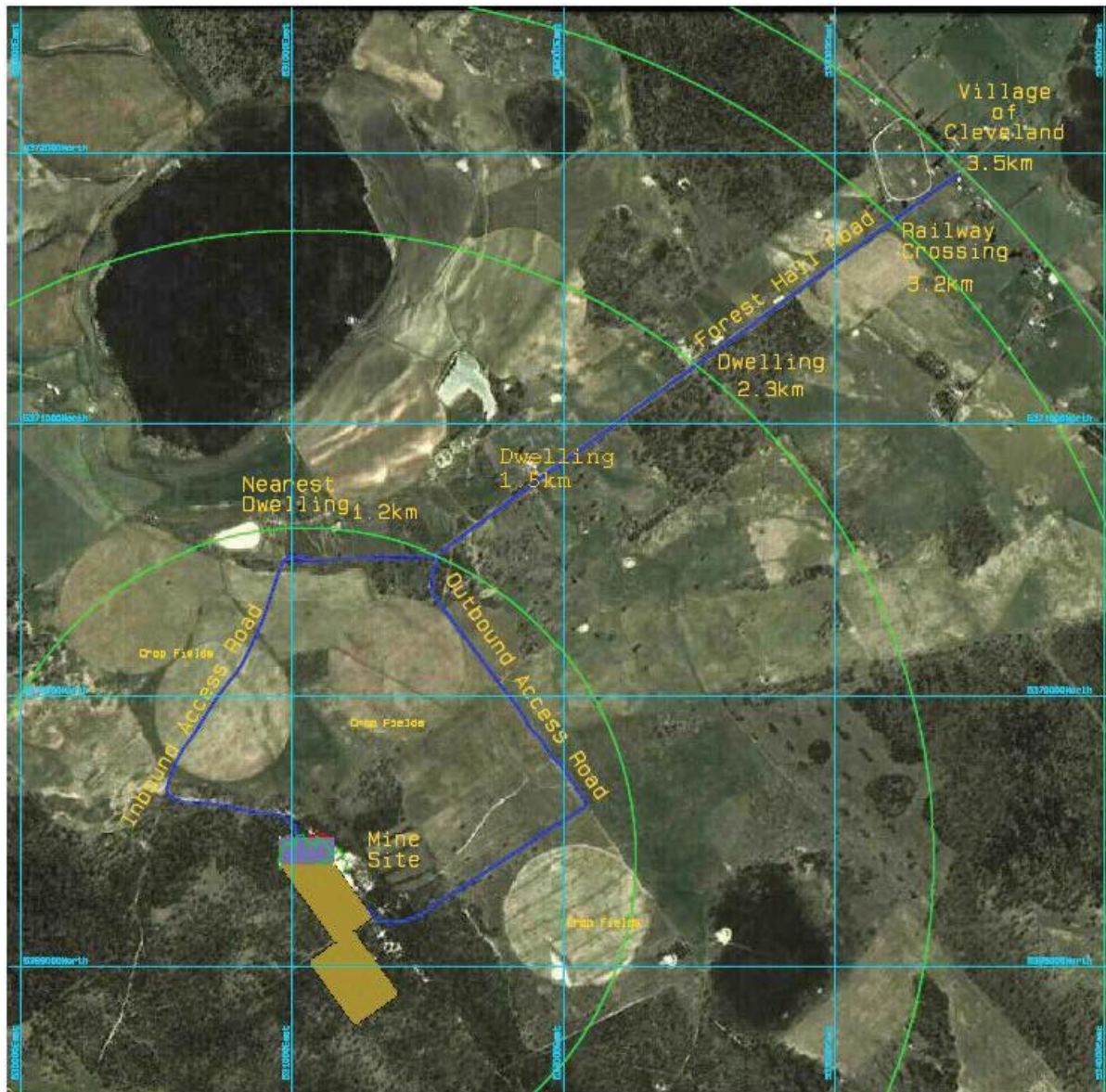
Figure 4: Proximity plan showing the inbound and outbound access road and nearby residential dwellings (sensitive receptors). The landowner's residence is located 1.2 km to the north and the nearest sensitive receptor in other ownership is located approximately 1.5 km to the northeast of the Activity Area (adapted Figure 6 of the EER).
