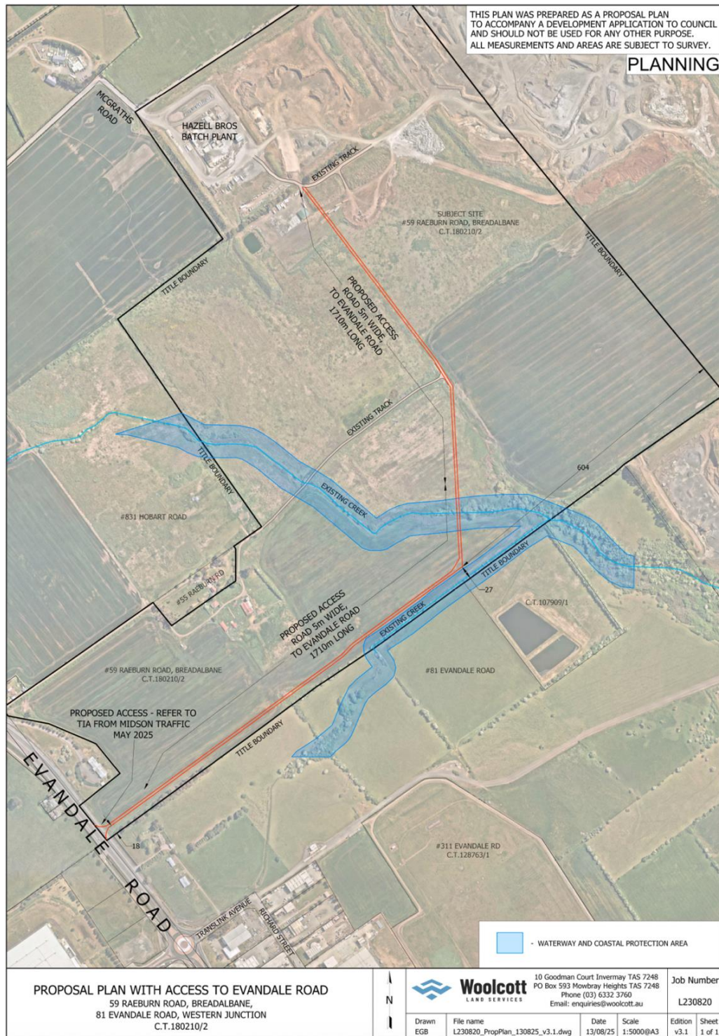
Figure 1: Site Plan showing the proposed road and the Briarly Creek crossing.
