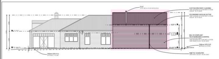
Image 4 Northern elevation with area of building envelope protrusion highlighted
