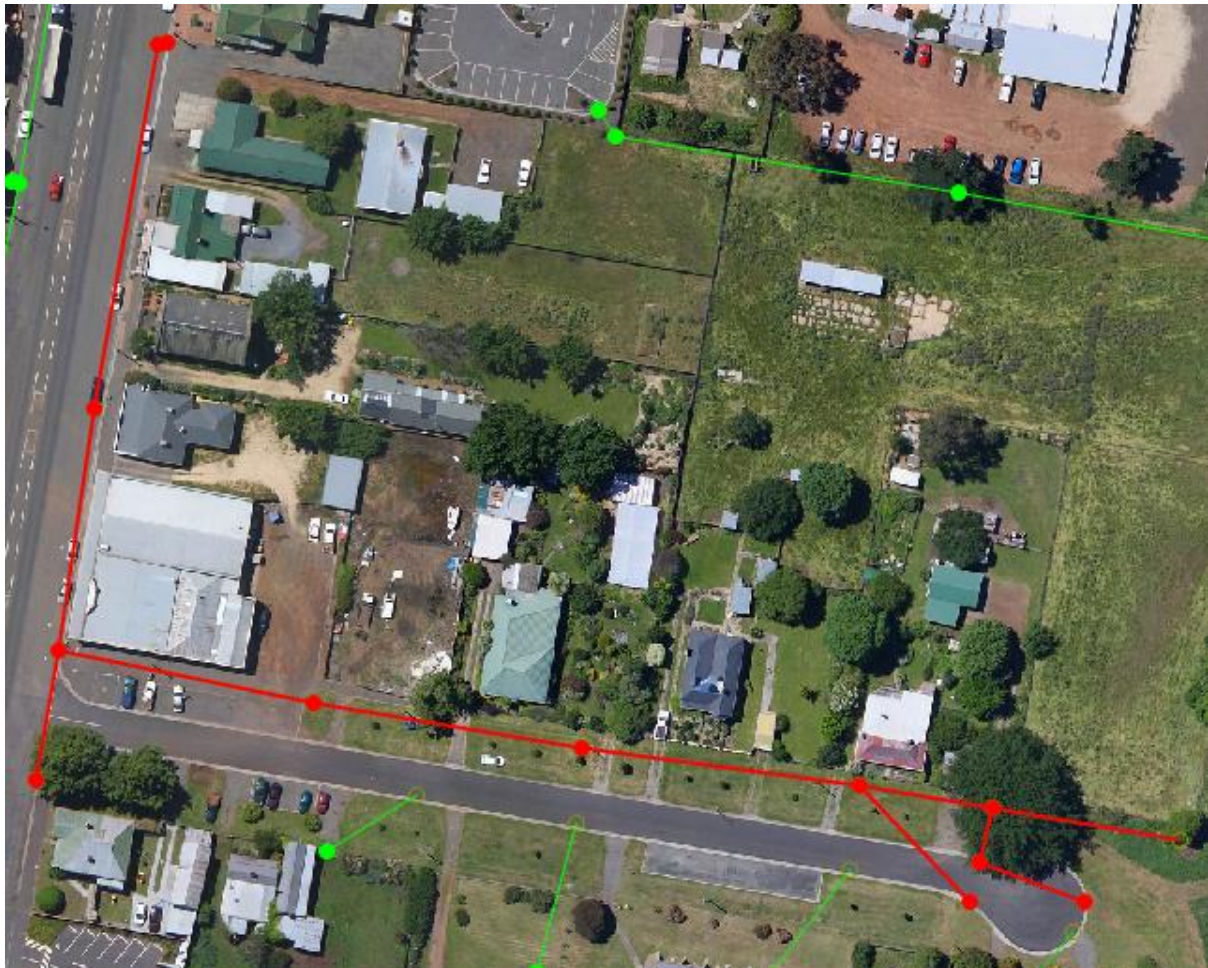
Figure 18. King Street stormwater system extent
