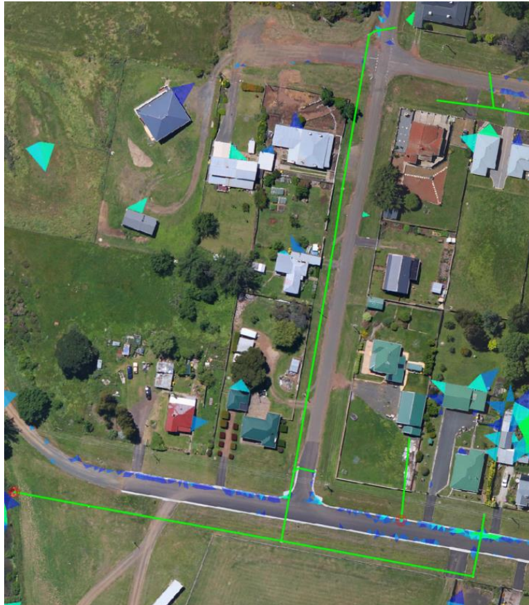
Figure 29. 10% AEP, 10-minute duration (storm burst no.10) (flooding >20mm deep)
