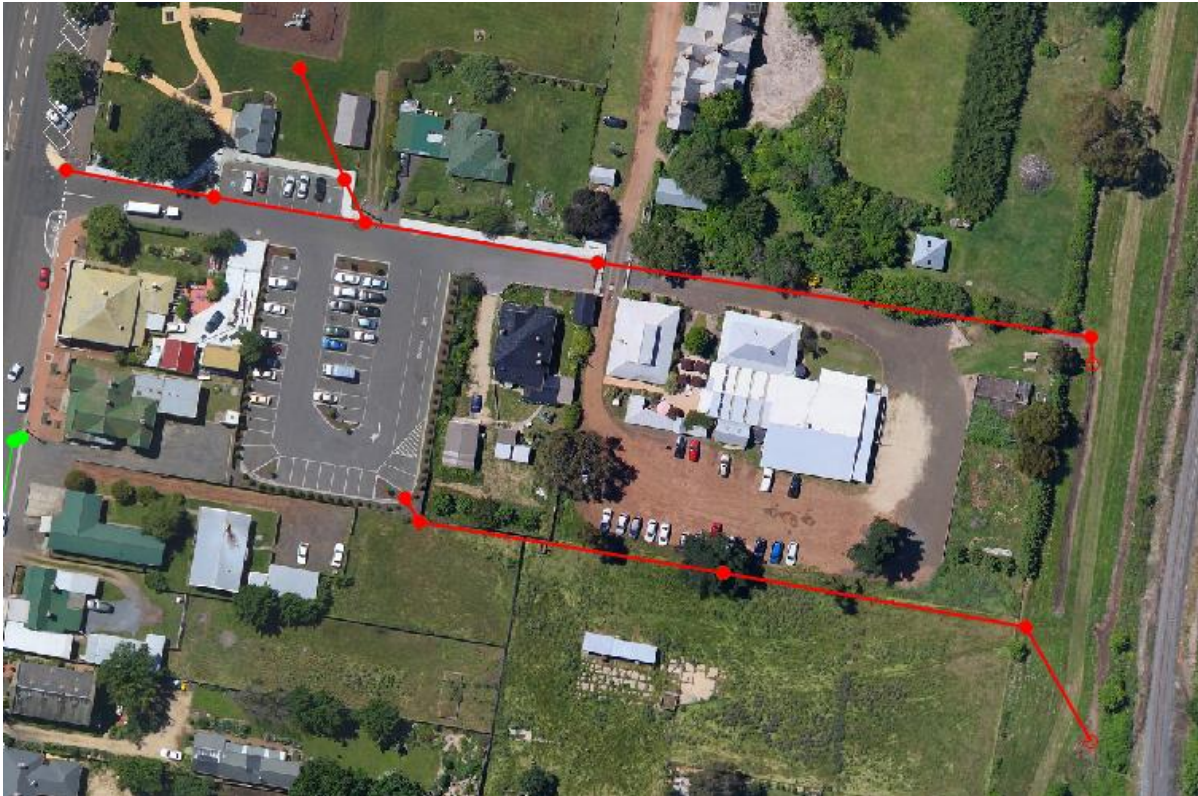
Figure 16. Commonwealth Lane subcatchment extent
