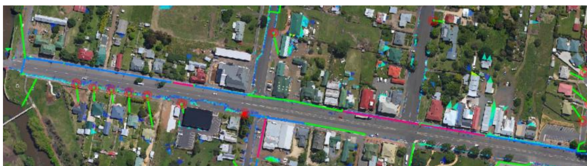
Figure 22. 10% AEP, 15-minute duration (storm burst no. 8) (flooding >20mm deep) (rotated 90 degrees)
