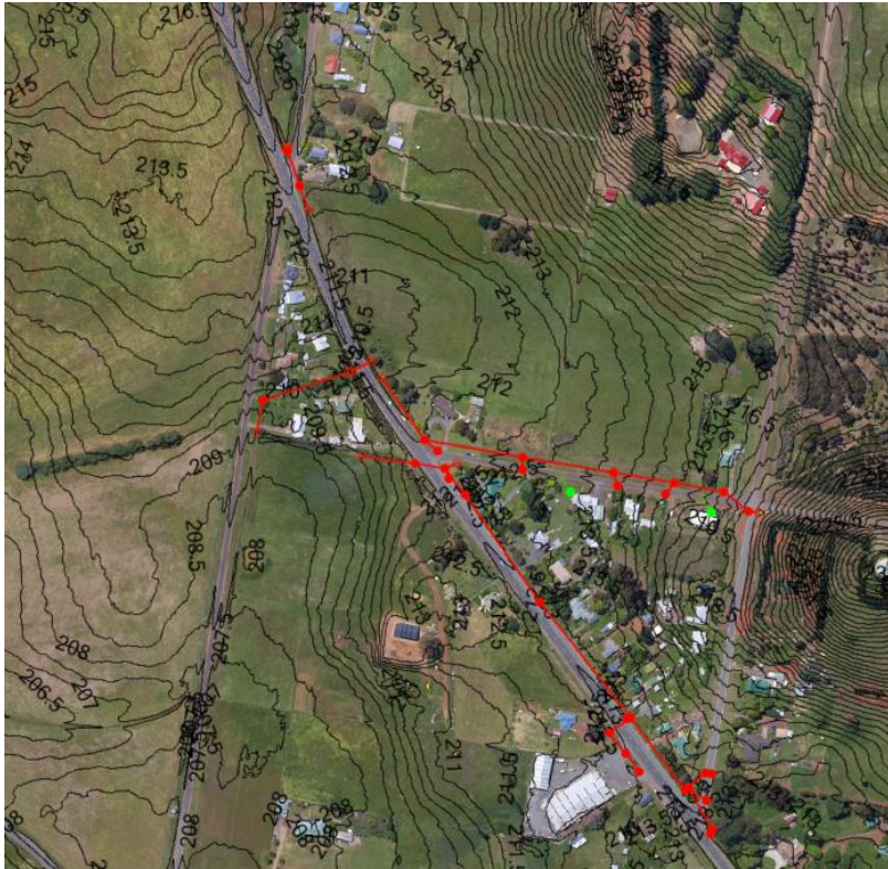
Figure 3. Hay Street stormwater system extent
