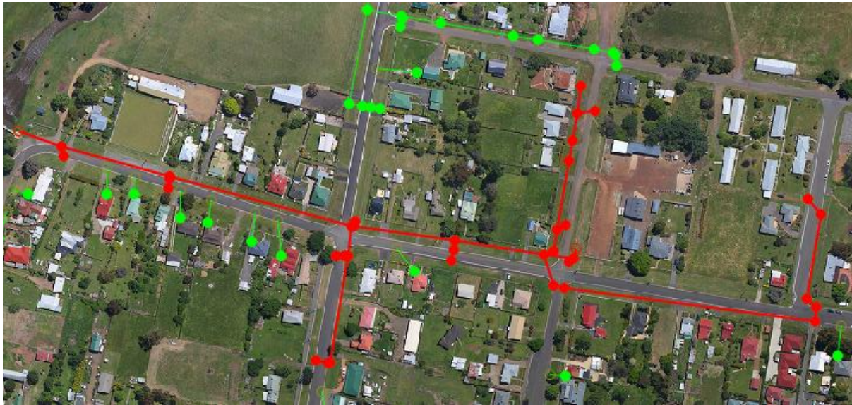
Figure 24. Bridge Street stormwater system extent (rotated 90 degrees)
