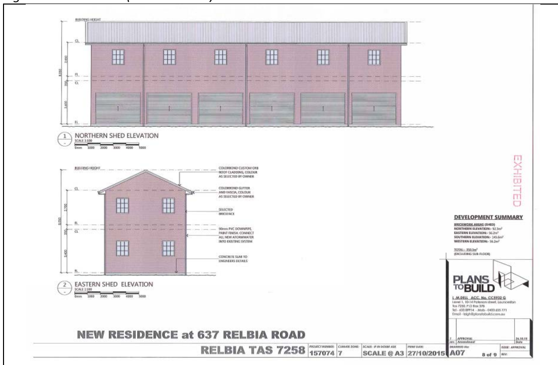
Figure 6 –Elevations (6 x 24m shed)
